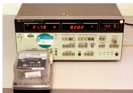
PHOTO 3: Testing the series impedance of the conventional electricity meter.
