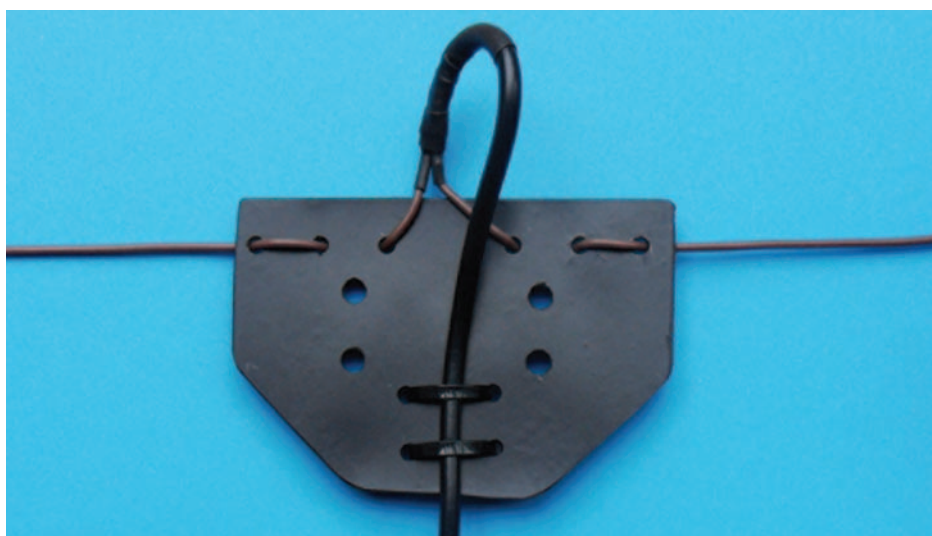
PHOTO 2: The HF antenna's dipole centre with 50Ω coaxial cable used to feed the antenna.
