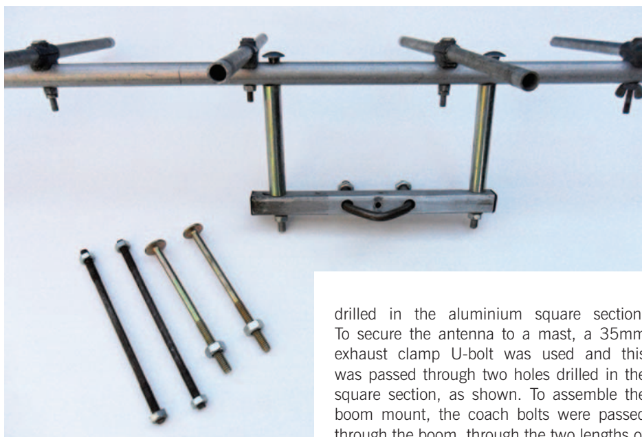
PHOTO 8: The boom mount constructed for the 70cm Yagi beam, plus some typical bolts that can be used (see text).
